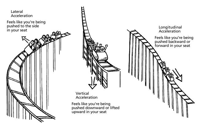
Accelerometers are calibrates in g's. A reading of 1g equals an acceleration of  $9.8 \text{ m/s}^2$ . As you live on earth, you normally experience 1g of acceleration vertically (no g's laterally or longitudinally). Listed below are the sensations of various 'g forces'. These are rough estimates, but may be helpful in estimating accelerations on the various rides.
