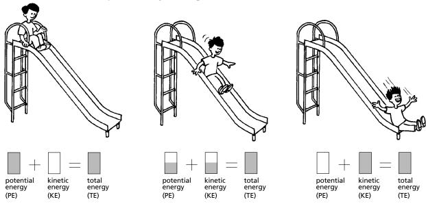
The diagrams above show the conversion of potential energy (PE) into kinetic energy (KE) during a slide ride.
